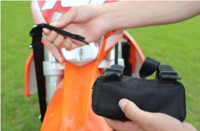
Thread the yoke through the pouch straps and the end of the pull strap (centre).
