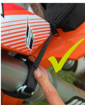
Ensure the angle of the centre strap is as flat as possible to minimize the load on the stitching (as shown in the pic on the left). The end of the yoke strap must end up on the inside of the fork, not on the outside as shown in the above pic.
