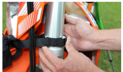
Thread the strap through the outer steel loop and run the strap back on itself pressing the velcro firmly together.
