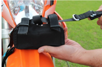
Thread the yoke through the pouch straps and the end of the pull strap (centre).
