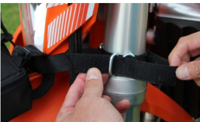
Thread the strap through the outer steel loop and run the strap back on itself pressing the velcro firmly together.
