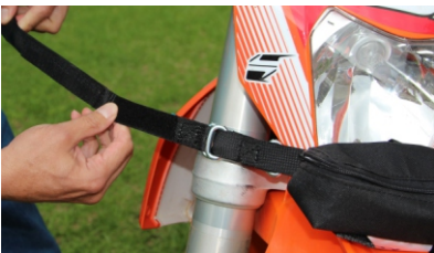
Repeat the process on the 2nd fork leg by running the strap round the outside of the fork, through the loop and back.
