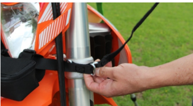
Run out the 1st side of the yoke around the outside of the fork leg, ensuring that the 1st velcro strip faces outwards.
