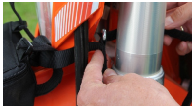
Turning the handlebar to full lock will help. Thread the strap end through the steel loop and bring it back.
