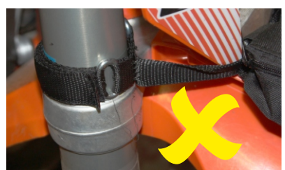
Ensure the angle of the centre strap is as flat as possible to minimize the load on the stitching (as shown in the pic on the left). The end of the yoke strap must end up on the inside of the fork, not on the outside as shown in the above pic.
