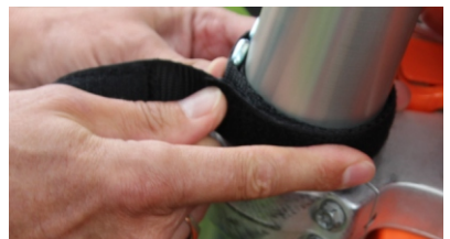
Be sure to press the velcro together firmly to ensure good adhesion.
