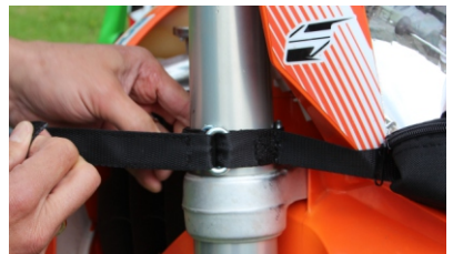
Repeat the process on the 2nd fork leg by running the strap round the outside of the fork, through the loop and back.
