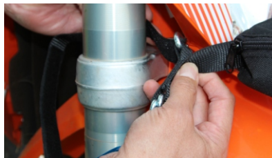
Repeat the process on the 2nd fork leg by running the strap round the outside of the fork, through the loop and back.
