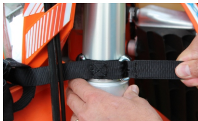
Thread the strap through the outer steel loop and run the strap back on itself pressing the velcro firmly together.
